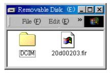
Remove the CF card from the card reader after confirming that the firmware update file "20d00203.fir" has been saved to the card.
