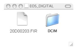
Remove the CF card from the card reader after confirming that the firmware update file "20d00203.fir" has been saved to the card.
