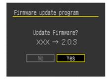
(4) Execute the firmware update after confirming the version to be installed, by selecting [Yes] with Quick Control Dial and pressing the "SET" button.
