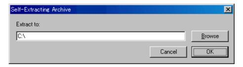
Clicking "OK" will cause the file's contents to be extracted and the firmware update file "20d00203.fir" to be created. (Click "Browse" to select a destination for the extracted files. This destination may be different from the path initially displayed, "C:")
